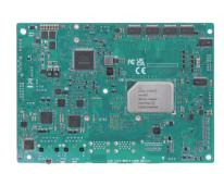
PEB-2274 is built upon Intel Atom® x6000E series processors (formerly Elkhart Lake). It features DDR4 memory up to 32GB, two Gigabit Ethernet ports, three M.2 sockets, and wide voltage of power input from 9V to 36V. It supports industrial temperature range from -40°C to 85°C, and can operate with TDP under 12W for fanless applications.
