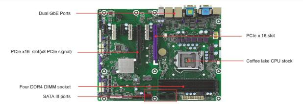
RUBY-D811 is based on Intel® Q370 chipset and Desktop processors including Intel® 8th Gen Core™ i3/i5/i7 SKU. This board supports DDR4 ,PCle 3.0, and SATAIII. Those fratures help you to build high performance and stabile system.
