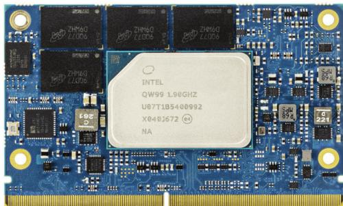
The new Engicam's SMARC standard module is based on Intel processors ELKHART LAKE series ATOM<sup>®</sup> x6000E (Pentium<sup>®</sup> and Celeron<sup>®</sup> available soon).
