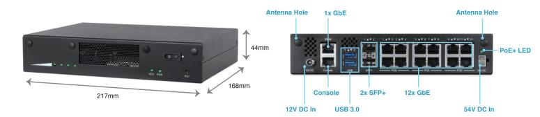
ANS-8A62/64 series builds on Intel® Denverton C3758/ C3558 processor with up to eight CPU cores. ANS Denverton series is a compact system with up to 2x SFP+, 13x GbE ports and PoE+ support, it is suitable for SDN (SD-WAN) application with 5G and IoT devices deployment.
