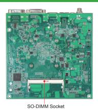
WADE-8079 is based on  $Intel^{®}$  Atom<sup>TM</sup> processor E3800 product family with memory and PCI Express controller integrated to support two-channel DDR3L memory and PCI Express 2.0 lanes. Portwell has taken advantage of such technology to furnish a series of products that meets multiple industrial requirements for cost effectiveness, reliable performance and a high level of data integrity and uptime.
