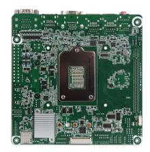
WADE-8212 is based on Intel® Q470E chipset and the latest 10<sup>th</sup> Gen Intel<sup>®</sup> Core<sup>™</sup> i3/i5/i7/i9 SKU. This board supports DDR4, PCle 3.0, and SATA III. Those features help you build high performance and stable system.
